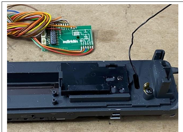
Fig 9 - Decoder holder mounted.
