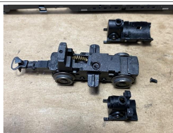
Fig. 3 - Old motor saddle (top) and new motor mount (bottom).
